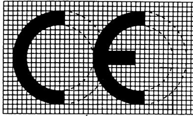
If the mark is reduced or enlarged the proportions given in the graduated drawing must be respected. The two letters of the CE marking must have substantially the same vertical dimension, which must not be less than 5mm. The grid does not form part of the mark and is for information only.
